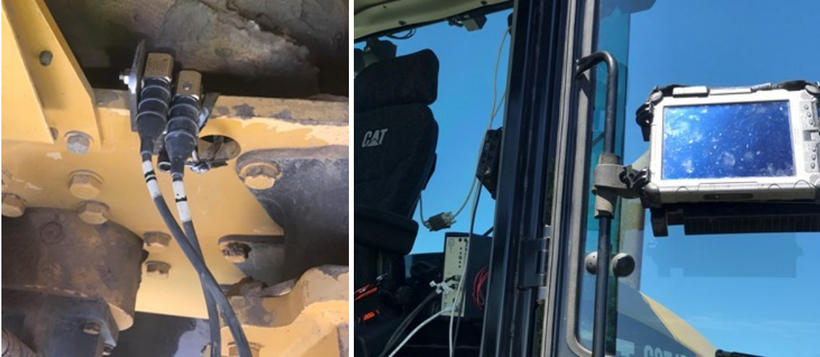
Figure 8. UTEP Moduli ICMV Accelerometer (left) and onboard display (right).
