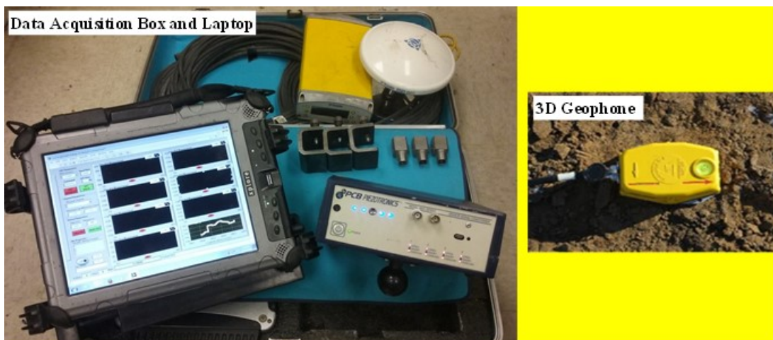
Figure 14. Geophones (left) IC calibration system (right) 3D geophone installation (Nazarian et al., 2020)
